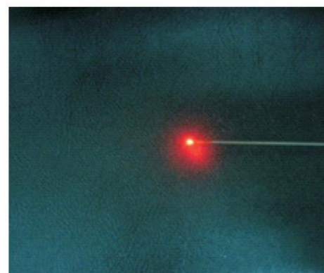
Fig. 4: Bright red aiming beam output for clear visualisation of the current position with a 300 \mu\text{m} fiber set during the treatment.
